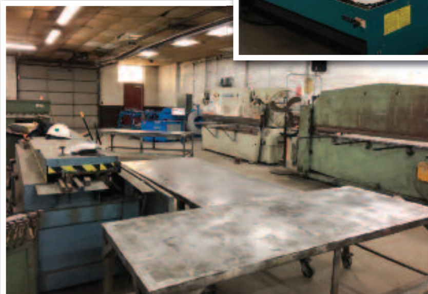
Spiral machine, brakes, and shop equipment
